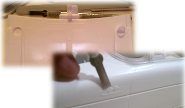
Ejector pin marks make removal difficult.
