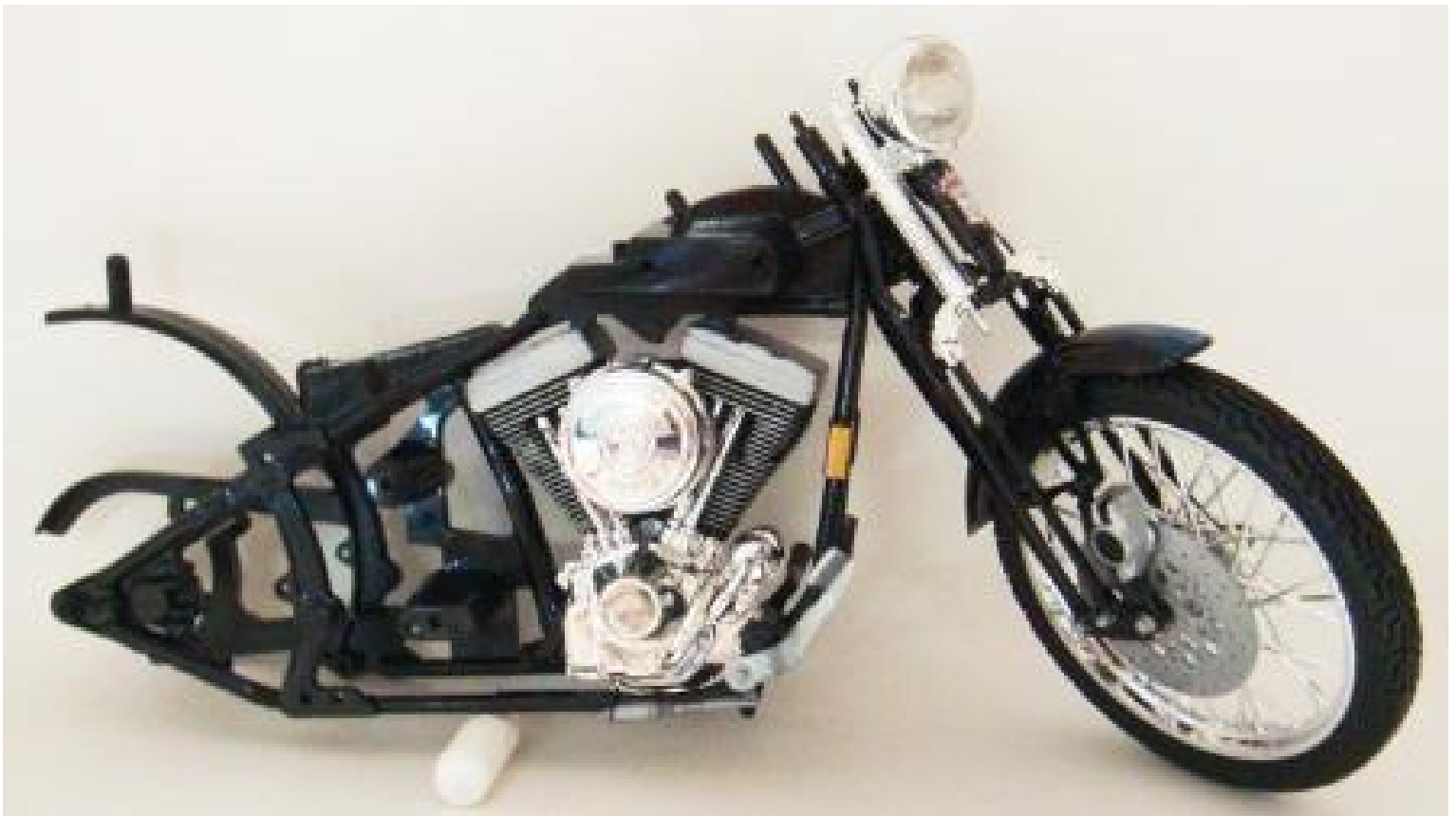
Figure 509 The headlight assembly and the front tire are installed onto the motorcycle frame.
