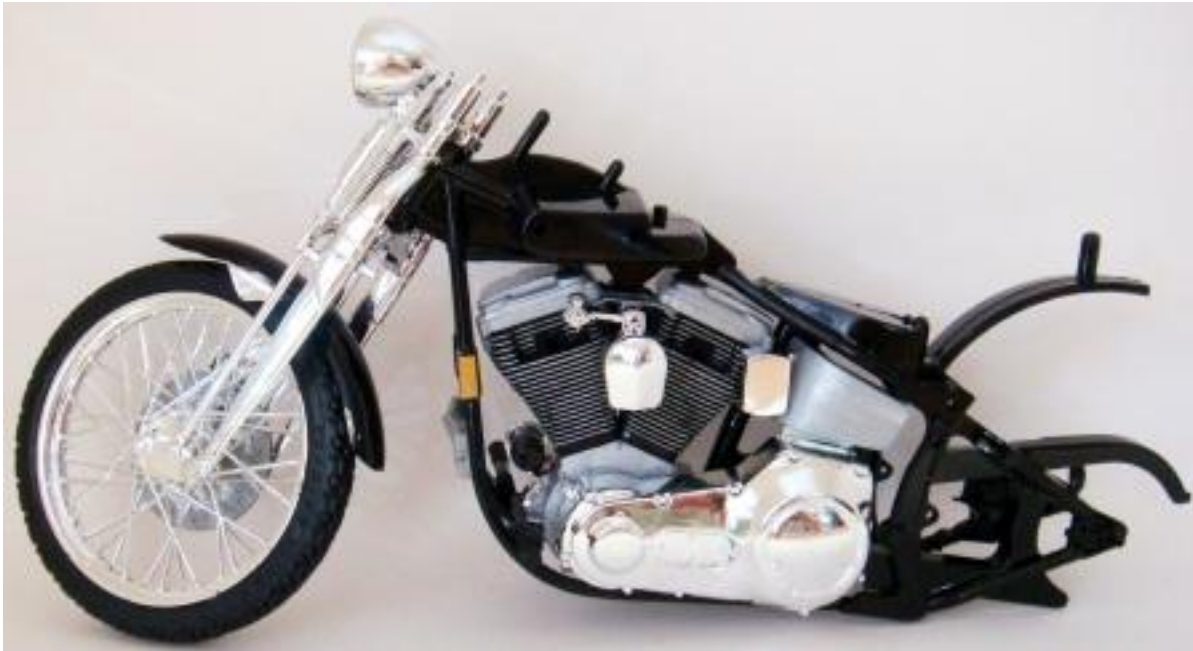
Figure 213 For Step 5 the Left Engine Half (Figure 205) is snapped into the left side of the motorcycle. On the Transmission Cover the oil tank is brush painted Testors Aluminum and then the Transmission Cover is installed into the motorcycle frame. Now the horn cover is snapped into place completing Step 5.
