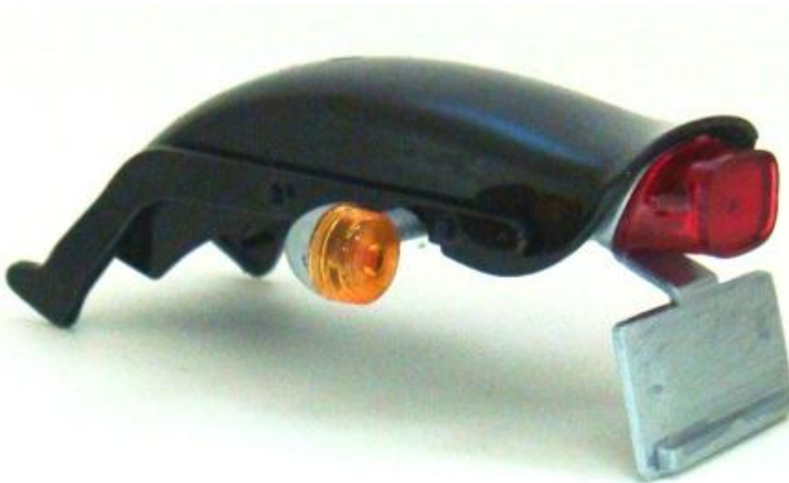
Figure 515 The Rear fender, left and right side brackets are spray painted Testors Gloss Black with the license plate bracket being brush painted Testors Aluminum. Both of the side brackets are snapped into the fender. The tail light and turn signals are installed onto the license plate bracket and then the license plate bracket is snapped into the rear fender.
