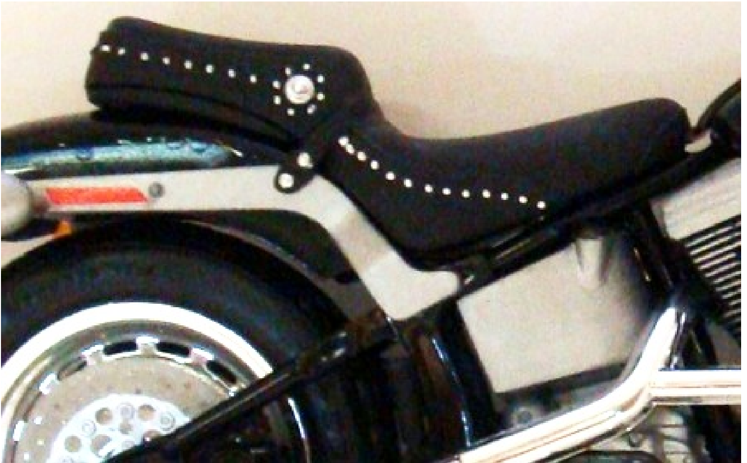
Figure 222 The seat and the seat bottom are both brush painted Testors Flat Black. The seat buttons are then brush painted Testors Silver. To install the seat the front of the seat is put under the instrument panel and then the seat bottom is snapped in place under the back of the seat and placed on a peg sticking up from the rear fender. A helpful hint is to use a jeweler's screwdriver to push up on the peg while pushing down on the seat.
