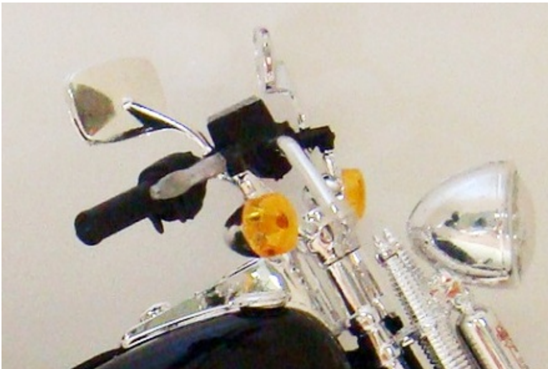
Figure 223 The handle bars are now assembled onto the motorcycle. The right and left hand grips are brush painted Testors Flat Black and then the brake levers are brush painted Testors Aluminum. The hand grips are then slid onto both ends of the handle bars. The turn signal lenses are put on the turn signal housings and then the assemblies are installed to the bottom of the hand grips. The left and right mirrors are then snapped to the top of the hand grips. The handle bar assembly is then snapped to the front forks.
