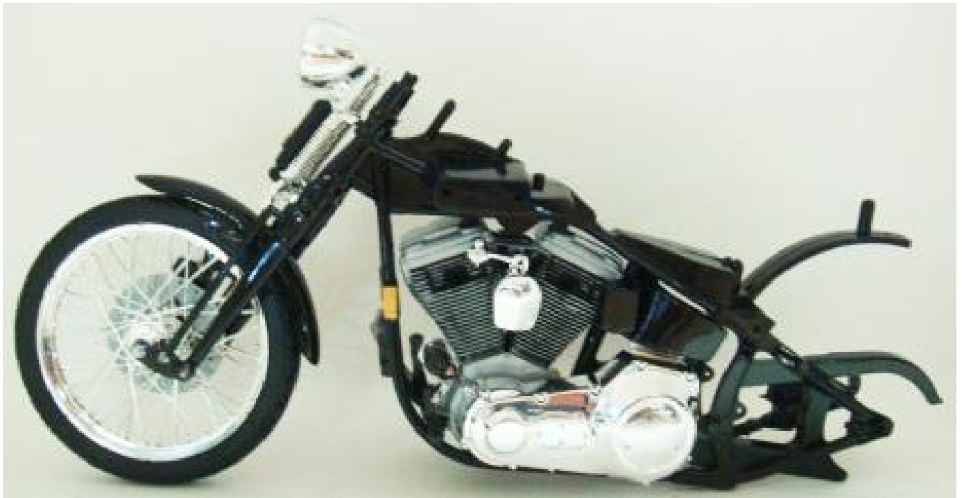
Figure 510 The left engine half Figure 503 is snapped into the left side of the motorcycle frame. The oil tank and coil cover part of the transmission cover is brush painted Testors Gloss Black and is installed into the motorcycle frame. The horn cover is then snapped into place between the engine cylinders.
