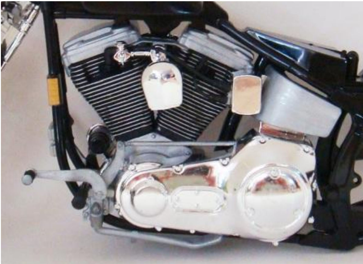
Figure 214 Step 6 is a very simple assembly. The pedal is snapped into position on the kickstand and the assembly is brush painted Testors Aluminum. The pedal also has the foot peg part brush painted Testors Flat Black. The assembly is then snapped into place on the left side of the motorcycle. Now the sparkplugs are installed in their positions.
