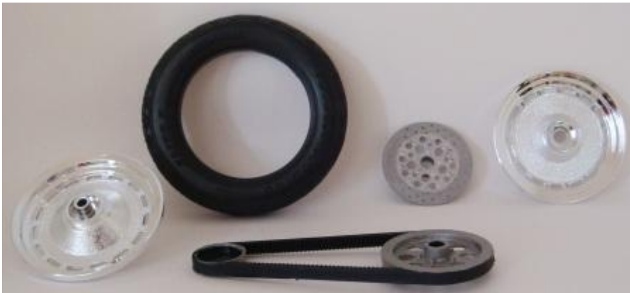
Figure 216 In this Figure all the components for the rear tire assembly; the rear tire, right wire wheel, left wire wheel, drive belt, and rear disc brake (Figure 211). The drive belt pulleys are brush painted Testors Steel and the belt is brush painted Testors Flat Black.
