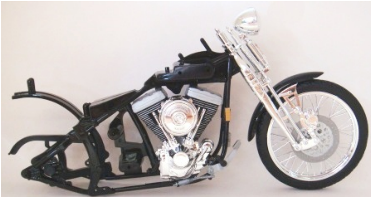
Figure 212 To complete Step 4 the headlight is assembled as well as the front tire. The headlight lens slides into a groove on both halves of the headlamp and then the headlamp halves are snapped together. The front tire assembly consists of; front disc brake (Figure 211), right side wheel, front tire, and left wire wheel. After the front tire is assembled it is installed into the front forks. The headlight assembly is then snapped onto the front springs, which is then snapped into place on the forks.
