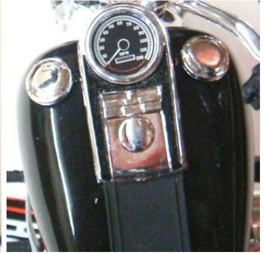
Figure 221 & 228 Decal 4 & 5 are applied to both of the gas tank halves and then the left gas tank half is installed followed by the right gas tank half. The odometer decal is applied to the instrument panel and then the instrument panel is snapped into place above the gas tank halves.
