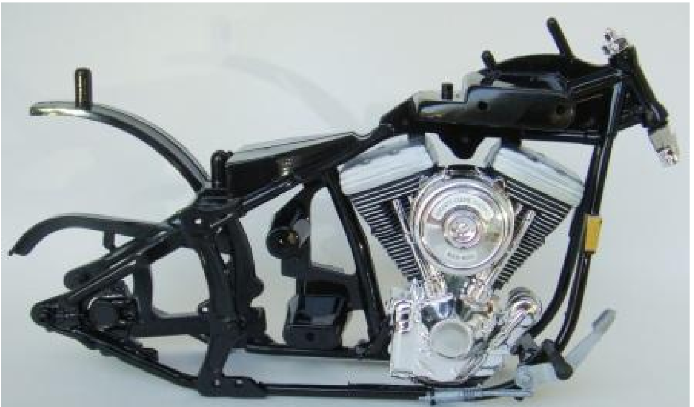
Figure 206 The foot pegs are snapped into position on both frames in the front area. The right engine half is then snapped into the engine area. Now the oil filter is brush painted gloss black and then snapped in place on the push rods. The push rod assembly is then snapped in place in front of the right engine half. This is followed by the air cleaner being attached to both cylinders on the right engine half. Decal # 12 is applied to the air cleaner. The foot brake is brush painted Testors Aluminum and Testors Flat Black before being snapped onto the frame and foot peg.
