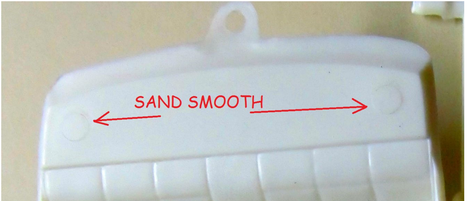
Pic 17 is a close up of the rear interior deck. Sand the injection mold pins smooth before painting. Interior Painting: Assemble the front seat and seat back before painting. Paint the outside of the interior tub Flat Black on the front part as it will show in final assembly. Paint the interior tub your main interior color.
