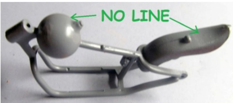
PIC 17 With the motorcycle frame in Primer you can carefully wet sand it and paint it with the rest of the parts. Notice the mold lines are hidden in the primer; the area on the fender where it shows will be under the seat so it won't matter.
