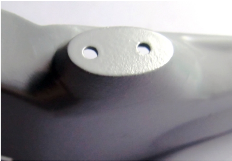
PIC 12 A good wet sanding with 800 grit paper should remove any blemishes and make the parts ready for paint coat. If needed apply more putty and repeat the process until you get the proper look as in the photo.
