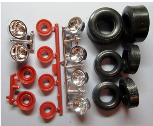
wish to make your car have a driven look use 220 grit sandpaper and roll the tires while pressing them on the paper. Paint the wheel backs Flat Black with a Silver rim. Install the rim fronts in place and slide the hub through the hole in the wheel backs until the back is flush in the tire.
