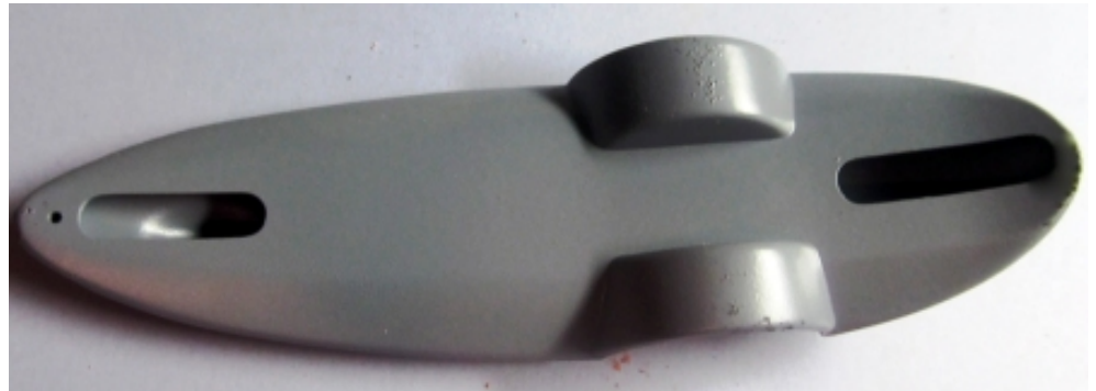
PIC 13 PIC 14 The trailer is the same color as the body so I did that at the same time. Assemble the two halves and wet sand the whole thing with 800 grit paper. Primer the trailer at the same time as the rest of the body parts as to save time.
