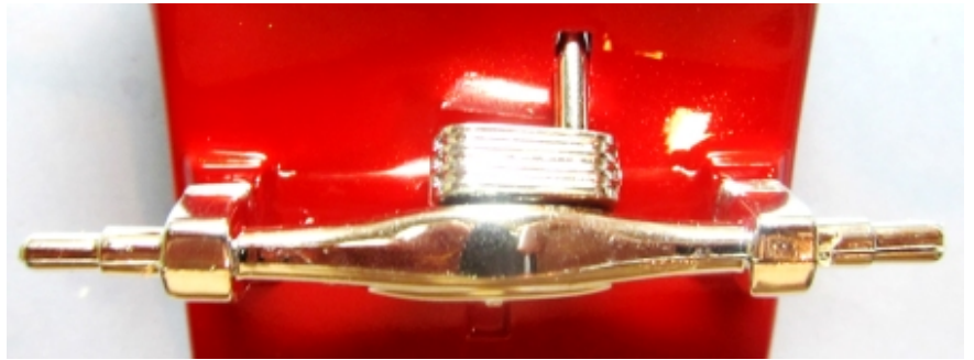
PIC 28 PIC 29 The front and rear suspension mount directly to the bottom of the body tub. Install the front axle in place and attach the radius rods to it and the indent on the body. Assemble the rear axle halves and add the transmission box. Install that unit in place on the back of the body tub.
