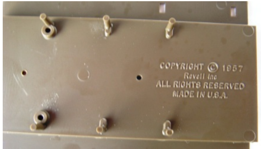
Figure 2701 and Figure 2702 For a competition build the copy right logos on the frame and the bed need to be removed. This can be done with a hobby knife and some sand paper. Revell did not update the copy right dates so the kits molds appear to be 57 years old.
