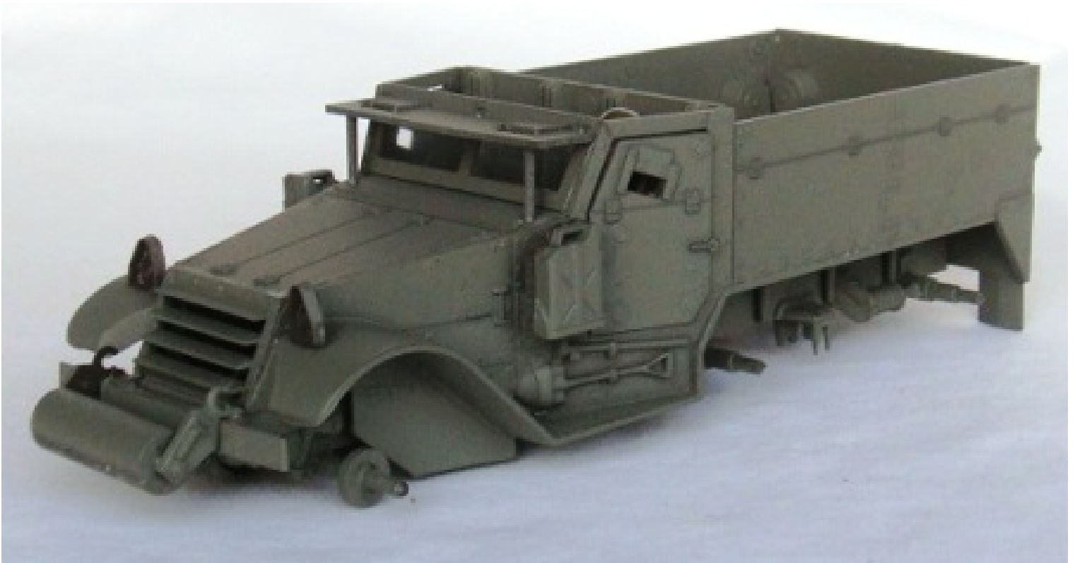
Figure 2723 The right and left head lights are installed onto the body assembly. The windshield armor is installed onto the windshield frame. The roller halves are glued together. The left and right roller brackets are attached to the roller assembly and then the roller brackets are glued to the front bumper.
