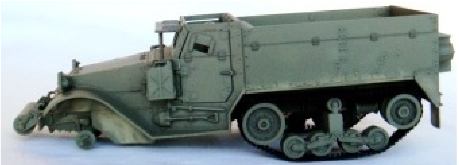
Figure 2728 The tracks are installed onto the inner drive wheel, inner idler wheel, and the bogie wheel assemblies. The outer drive wheels are installed onto the posts by the cab and the outer idler wheels are installed onto the posts by the rear panel section. The body assembly is weathered with sand from Tamiya Weathering Master Set A.
