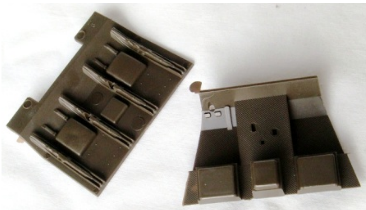
Figure 2705 There was flash on the floor board and the rear cab wall. This can be easily removed with a hobby knife.
