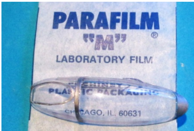
Pic 37 & 38 After the canopy ribs were dry I used some Parafilm frisket to mask the canopy. Simply stretch it on and tuck it under the whole thing. This is known as frisket film and you can find it at a hobby store.
