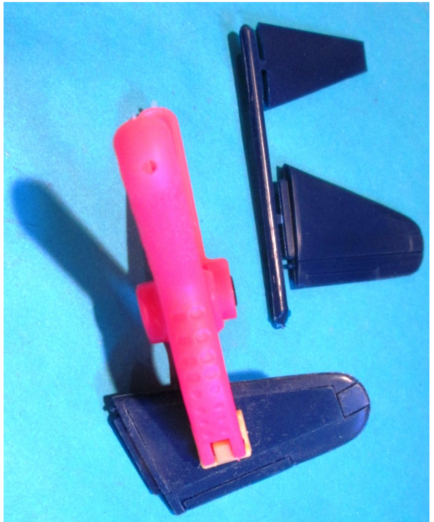
Pic 29 & 30 When test fitting the two-piece stabilizers together, I noticed the locating posts made the insert set too high. Remove the top part of the post with a hobby knife or rotary grinder. They position well without the post and after applying some tube glue just place a light duty clamp on it to keep them in place while they dry.
