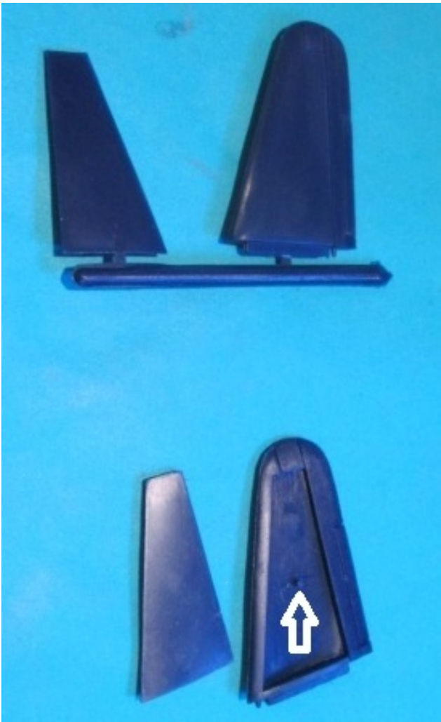
Pic 29 & 30 When test fitting the two-piece stabilizers together, I noticed the locating posts made the insert set too high. Remove the top part of the post with a hobby knife or rotary grinder. They position well without the post and after applying some tube glue just place a light duty clamp on it to keep them in place while they dry.
