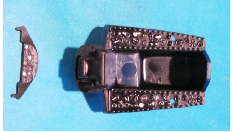
Pic 13 & 14 The gauge decals that are included in this kit don't fit the small instrument panel at all. I painted it flat black and picked out the individual gauges with a toothpick and some white and silver bottle paint. I did the same to the cockpit console switches and gauges after an overall coating of flat black had dried.
