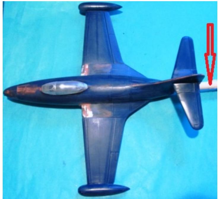
Pic 41 Go over the entire airframe looking for places that need some attention and then mount the plane on a 3/8" towel fitted to the tailpipe for priming.
