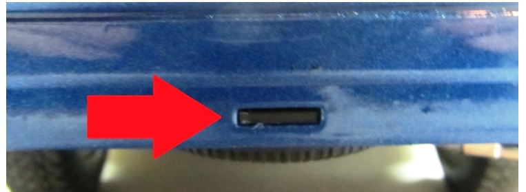
PIC 32 PIC 33 Attach the chassis to the body. There are pins in the front of the chassis that line up in the front bumper. There is a tab in the back that attaches below the tailgate.
