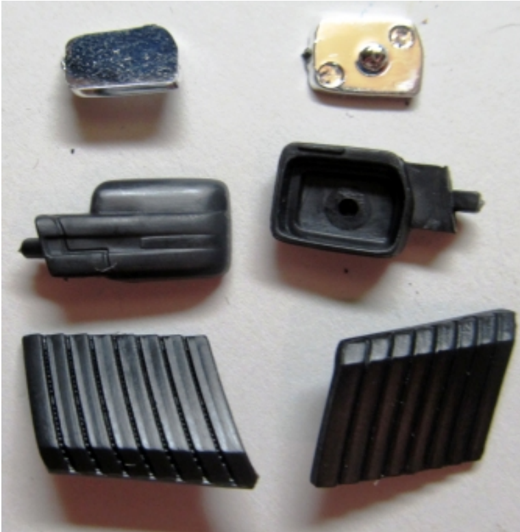
PIC 36 PIC 37 Finish the assembly by painting the top half of the mirrors Body Color and add the mirror faces. Install the mirrors. Install the hood vents. As they were the proper finish and color I did not paint them.
