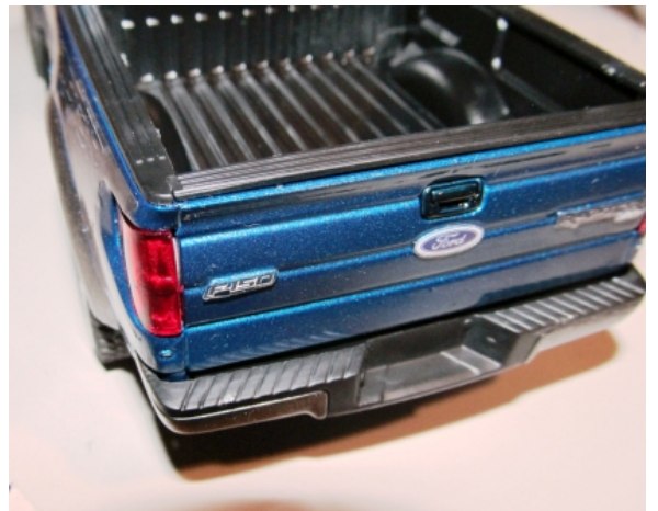
PIC 34 PIC 35 Assemble the bed caps and bumper. The tail lights snap in place. A little Elmer's Glue will hold them better. Paint the lower part of the bumper Gunmetal. Attach the bumper. The knob on the tailgate panel is Yellow. The tailgate panel is slid in place in the bed and the bed caps and tailgate cap added. As the Black was the correct finish and color I did not paint the parts.
