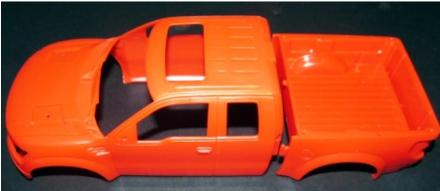
PIC 17 The body is in two parts, the cab and bed. To prepare the body for paint it needs to be wet sanded with 800 grit sandpaper. I found no blemishes or mold lines to remove on my sample.
