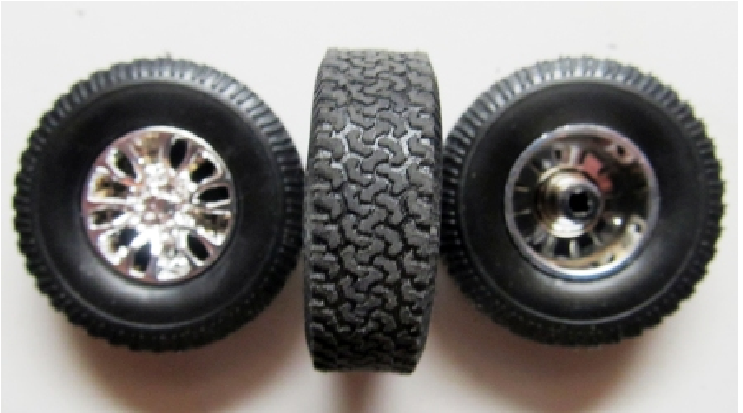
PIC 7 Give the tire a "Road Worn" look by pressing and rolling the tread on a sheet of 220 grit sandpaper.
