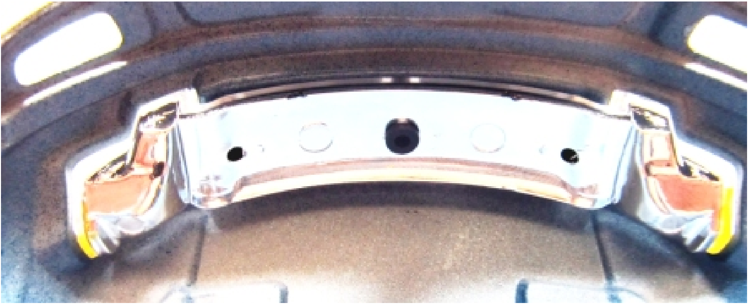
PIC 28 Install the lens and bezel units from the inside. Add the grille from the outside and press in place.
