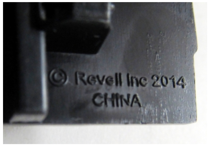
PIC 3 PIC 4 The chassis pan needs painting and detailing. Use different shades of Silvers, Aluminums and Steels on a Flat Black surface and detail as to your skill level. There is a Copyright Script on the rear corner that needs to be removed by sanding it smooth. Paint the brakes Silver with Gold calipers. Paint the mount area of the chrome tips Flat Black and install them.
