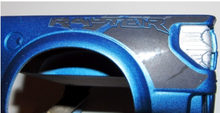
PIC 22 NOTE: If you prefer to do this after you clear coat the body do so. I prefer to add the stickers so it will be under the clear so they will never lift as they age and dry out. Add all the stickers to the tail gate, doors and bed side. I deleted the hood sticker in my build, add it if you wish. Now you can clear coat the body as normal.
