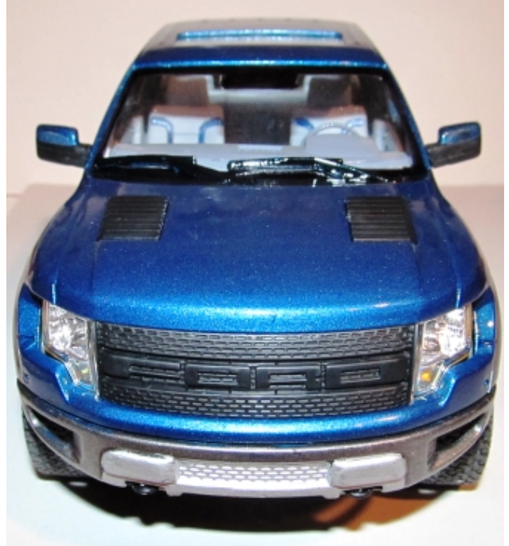
PIC 36 PIC 37 Finish the assembly by painting the top half of the mirrors Body Color and add the mirror faces. Install the mirrors. Install the hood vents. As they were the proper finish and color I did not paint them.
