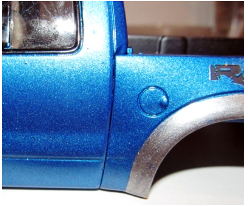
PIC 30 PIC 31 Line the bed up and snap it in place on the cab. Once finished, the body lines will match and the cab and bed will be very close.
