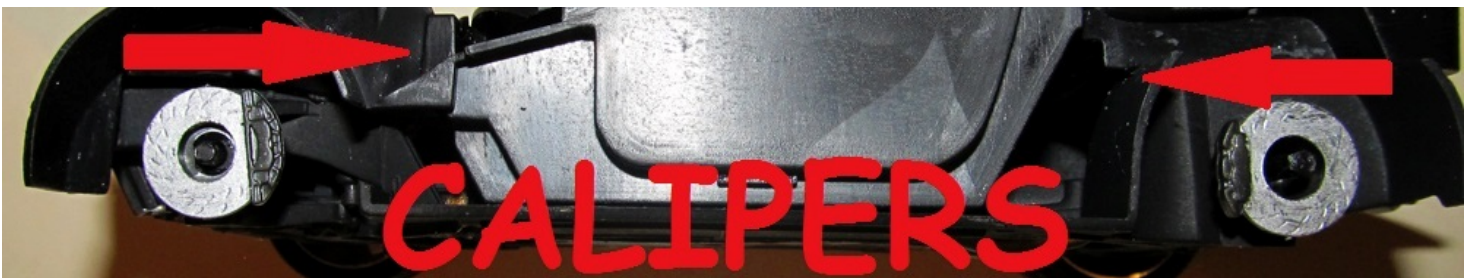
PIC 24 Insert the brakes onto the chassis with the calipers facing into the center. Add the metal axle.
