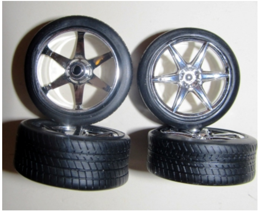
PIC 22 Using 220 grit sandpaper press and roll the tire tread on the paper to rough up the tread surface giving the tire a used worn look. Install the tires onto the rims.
