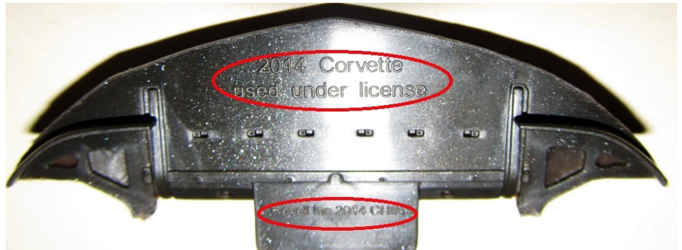
PIC 34 PIC 35 Assemble the hood with the vent and hinge. Paint the grille Flat Black. Note the Copyright needs removed from the bottom pan and it is painted Flat Black.
